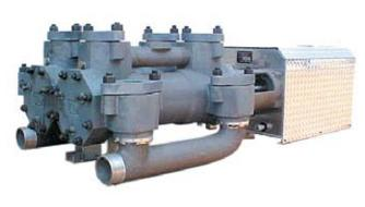
hydraulic-drive piston pump is rated 180 gpm at up to 325 psi, and 150 gpm at up to 800 psi. The 7.5-inch-by-10-inch duplex hydraulic-drive piston pump is rated 300 gpm at up to 800 psi, while the 7.5-inch-by-10-inch triplex hydraulic-drive piston pump is rated 450 gpm at up to 800 psi.
