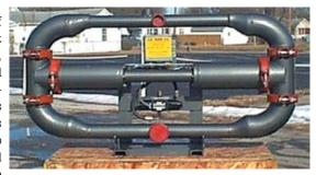
side (not flash-chromed), which helps provide very long life on the chambers. The company has had thousands of the grout pumps in the field working since 1989, and mud pumps as reliable. Mud pumps are available from 20 gpm to 230 gpm, with pressures to 400 psi, and grout pumps to 2,000 psi.
